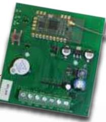
**RICEVITORE LINK-R4 (decoder 4 CH)**
